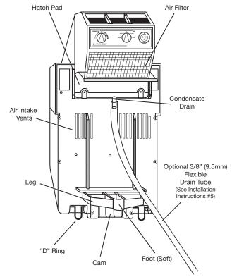
Figure 4. Bottom View of Carry-On
