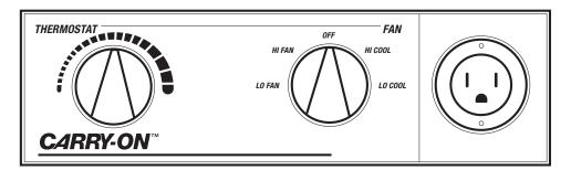
Figure 7. The Carry-On Control Panel
