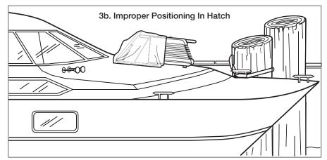
Figures 3a & 3b. These figures show proper and improper positioning and leveling of the Carry-On unit in the boat hatch. It is very important that the Carry-On be level.
