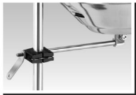
Round Rail Mount BOTH MOUNTS BELOW FIT ANY ANGLE RAIL Fits Standard Round Rail 1/2" or 1" (25mm or 25mm) Model 158923 A10-080 (MAGMA) Fits Oversized Round Rail 1 1/8" or 1 1/4" (28.5mm or 32mm) Model 437137 A10-085 (MAGMA)
