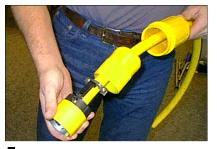
**5** Lubricate mouth of boot and rear shoulder of device with soap solution and pull into place.
