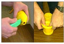
1 Cut boot at first line, if cord is greater than 5/8". Invert tapered end of the boot and apply soap solution.
