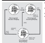
Press the [S/S] Button to Start the Chronograph (start counting) Press the [S/S] Button to Stop the Chronograph (stop counting) The elapsed time will appear on the display Repeat the above steps to resume counting and get the accumulated elapsed time (the time the Chronograph is stopped will not be counted when the chronograph resumes counting. To count total time from when Chrono starts and record laps or split times. use Lap Mode instruction in next section)
