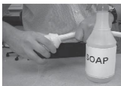
2. Apply soap solution to boot end and invert by pushing cord end against boot end. Push cord about 12" through boot.
