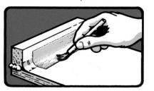
The fiberglass tape can be used to patch cracks and holes, or provide abrasion resistance to wear points such as stems and keels or the edges of paddle blades and centerboards.
