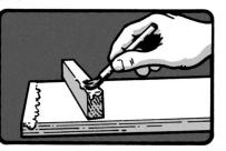
**2b** HARDWARE BONDING Before bonding hardware, pre-wet porous fastener holes using the pipe cleaner.
