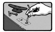
3 Thicken the remaining epoxy by stirring in filler until it reaches the desired consistency. The mixture should be thick enough to fill gaps between mating surfaces without sagging. The more uneven or wider the gap, the thicker the mixture should be. The mixture may be thickened to a very thick, peanut butter-like consistency for maximum gap filling or for filling and shaping low area or filling holes.
