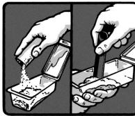
Apply epoxy, assemble and clamp parts within fifteen minutes. Working and cure time will be shorter in warmer temperatures—longer in cooler temperatures.
