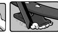
6a Add extra reinforcing to a joint by applying fiberglass tape over the fillet. Trim tape to the appropriate size then use the brush to saturate the fabric with epoxy and smooth the fabric in place.
