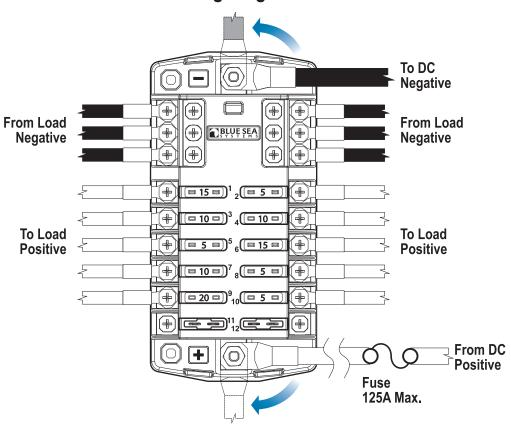
Application Note: This device is intended for branch circuit protection. Suitable main circuit protection of not more than 125A rating should be provided ahead of this device with an interrupt current rating consistent with the battery capacity. Consult ABYC E-11 Table V. See "Circuit Protection" at www.bluesea.com.
