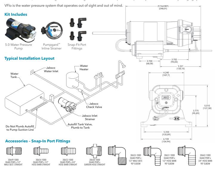
**NOTE:** Do not install VFlo with an accumulator tank. VFlo was designed to operate independently and will not function properly if paired with an accumulator tank.
