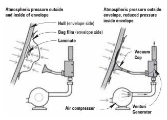
Figure 1—Typical repair before and after vacuum is applied
