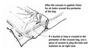
Small leaks in the bag, seal or mold will have a cumulative effect of reducing vacuum levels under the bag. Seal all leaks with sealant or tape to improve vacuum levels. Some materials such as press board are porous enough to not be suitable as a mold surface unless they are coated and sealed with epoxy.
