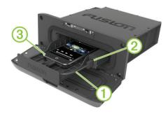
4 Connect the adapter cable to the media player ③, and place it in the device tray.
