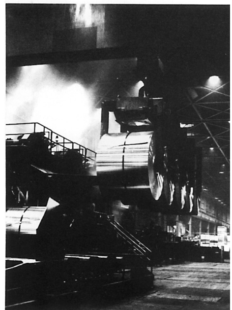
MANSAYER Style G1362, Multiple Gang, Telescoping, Leg Coil Lifter
