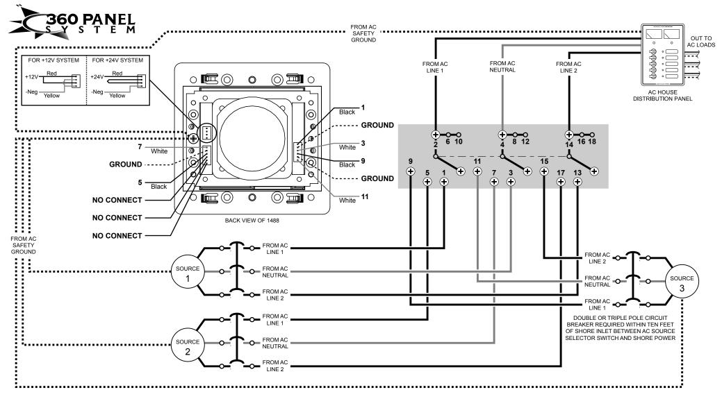
Warning: Do not cut out resistors in wire harness.
