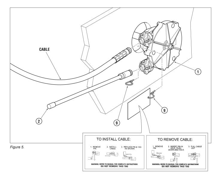
**STEP 3.** Replace pin as shown in Figure 6, making sure that it is fully seated. If pin cannot be inserted, the cable is not fully seated in the helm. Push on cable to ensure that it is fully home. **DO NOT REMOVE TAG FROM PIN.**
