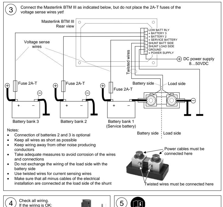
Install the 2 A-T fuses of the voltage sense wires
