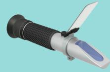
A refractometer measures the approximate freeze point of an antifreeze blend or dilution to check whether it is within manufacturer's specs. It does so by measuring the refraction of active ingredients within a mixture.
