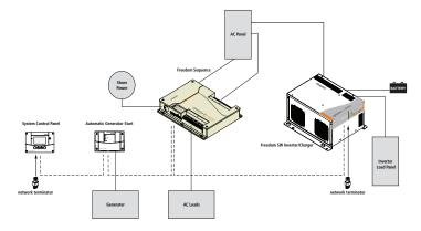
Figure 2 Typical Xanbus System Diagram
