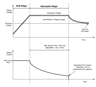
Figure 36 Two-Stage Charging Cycle
