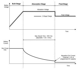
Figure 35 Three-Stage Battery Charging Cycle
