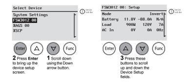
1.Typical device ID for a single installed Freedom Inverter/Charger. The second unit has a device name **FSW3012** is followed by **01**.
