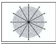
Bird Spider Arm "tips" should overhang mounting surface by at least 2".
