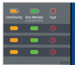
Battery fault detection LEDs
